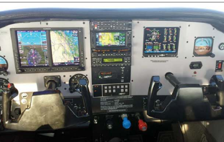
Spirit Avionics' demo panel currently includes: Mid-Continent Instruments and Avionics Lifesaver electronic ADI; Garmin G500 with synthetic vision & JeppView, GTN 650, SL 30, GMA 350, GTX 327, GDL 88, Century 2000 AP with altitude preselector and flight director; EDM 930 engine monitor; and more.
