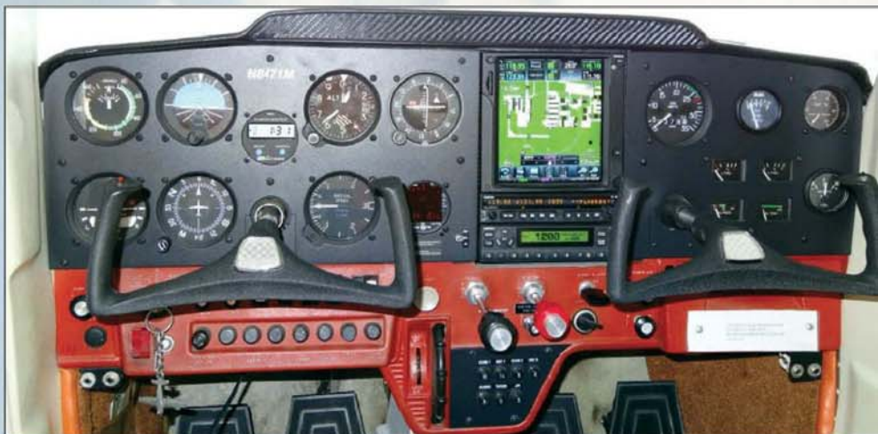
Tech Aero's demo panel currently includes: Garmin GTN 750, GMA 35, GTX 330, SL 30 and a JPI EDM 700 with fuel flow.
