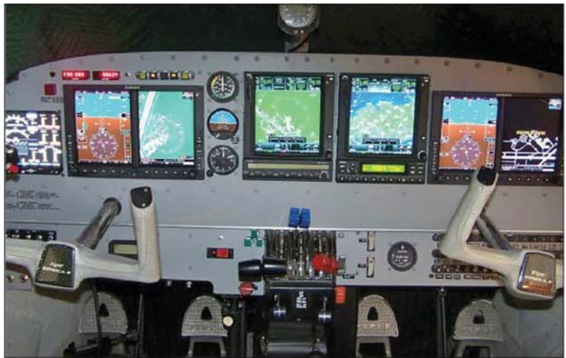
Gulf Coast Avionics' demo panel currently includes: dual Garmin G500s, dual GTN 750s, GDL 69, GTX 328, GTX 32; JPI EDM 960 engine analyzer; Avidyne TAS605 traffic, Cobham/S-TEC 55X autopilot; L-3 WX-500 Stormscope; and more.
