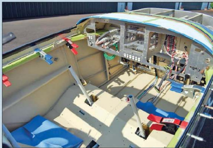
When completed, Pacific Coast Avionics' RV-7's panel will include: Advanced Flight Systems' two-screen EFIS with engine monitoring; Advanced/TruTrak autopilot; Garmin GTN 750, GNC 225A, GMA 35, GTX 33, GDL 39; Vertical Power VP-X Pro; and more.
