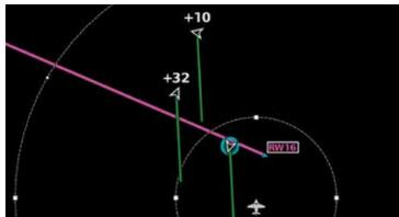
To enhance flight safety, TargetTrend relative motion technology offers pilot a faster, more intuitive way to judge the direction and closure rate of traffic targets in relation to the aircraft's position.
